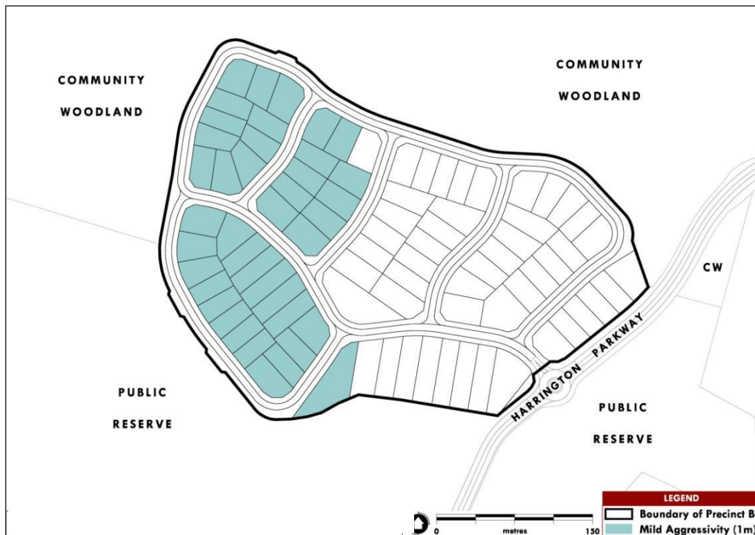
Figure S4-24: Aggressivity to Concrete and Steel in Precinct B
